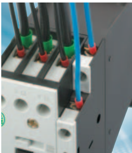
Figure 9: Now the coil connections are located at the front of the contactor. Since, therefore, they are no longer obstructed by the often rigid main current cabling, wiring and voltage testing is simpler and takes less time. The second level contains the connections to the integrated auxiliary contact.
