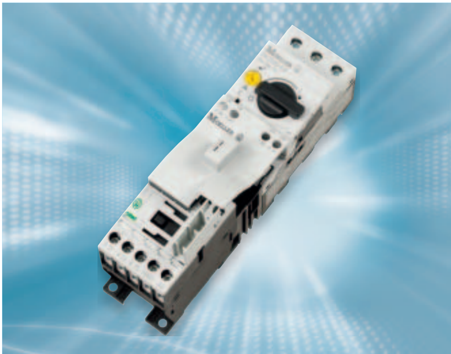
Figure 17: Tool-less plug-in connection technology on a direct-on-line starter with the advantages of secure fixing on just one carrier rail and positive and error-free connection between motor-protective circuit-breaker and contactor. The physical volume of the mechanical link is used for ancillary functions of the tool-less plug-in connection technology in a further development stage of the system.
